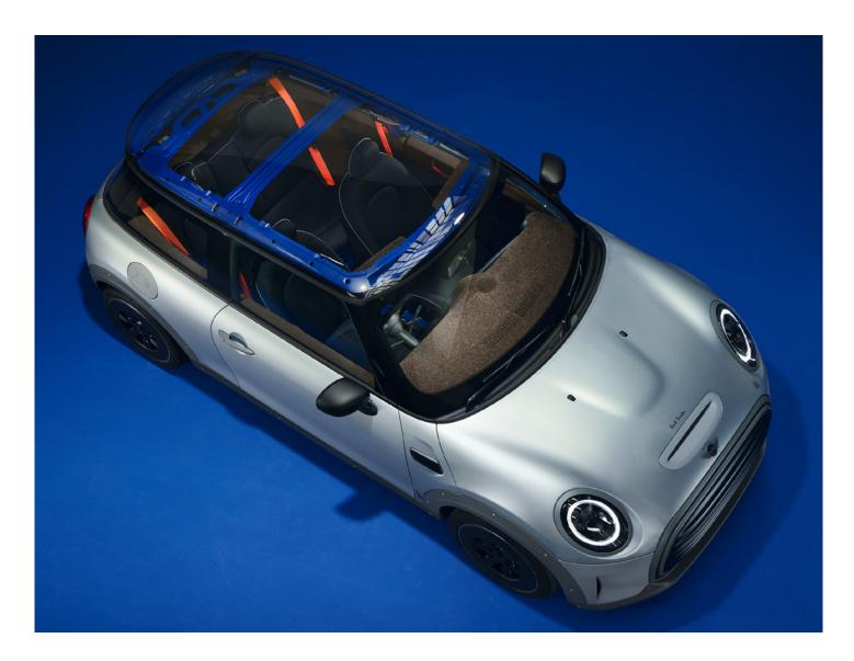
Integrated within the top of the car's dashboard, sun visors and doors, cork is a natural raw material, that helps reduce the environmental footprint of the German manufacturer's new prototype, designed by the British stylist, Paul Smith.
