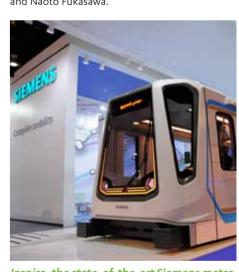
Inspiro, the state-of-the-art Siemens metro Inspiro, the surface metro recently launched in Poland by Siemens, is the most modern and sustainable in its class. With a modern design, cutting-edge technology and an environment--friendly concept, it is one of the lightest metros in the world as a result of the installation of the innovative AluCORK cork flooring, which contri-butes to a 30% reduction of the carriages weight.
